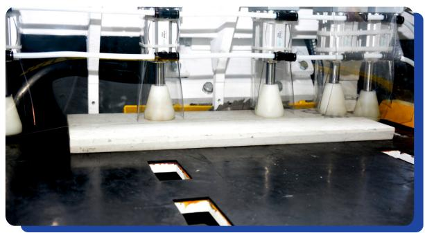
The more accurate cut, the better result. With the GM45 MitreSaw, an accurate mitre cut is achieved each and every time due to the fixed 45.0° angle of the cutting blade and the straight edge system which uses the front edge stopper of the material to position it accurately on the table. No measuring. No mistakes.
