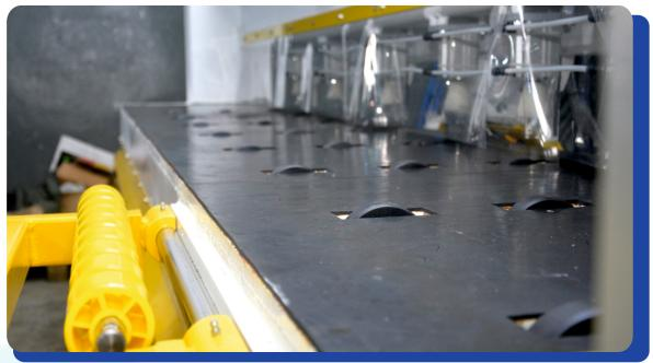
The GM45 MitreSaw's reputation for accurate cuts is also due to fact the material is loaded polished face down, there by eliminating cutting errors that can arise due to small variations in material thickness along its length.
